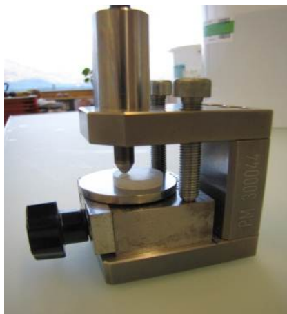
Fig. 9a Setup for the crack initiation test
